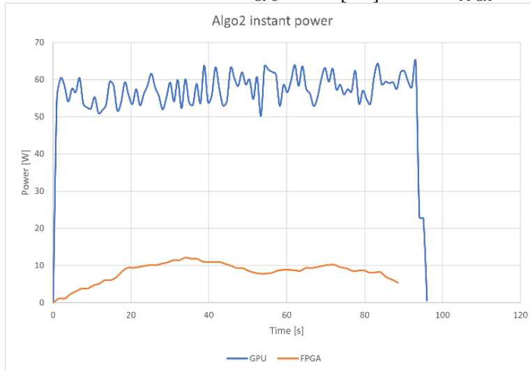
Fig.18 P_A(t) for ALGO2 executed on FPGA and GPU when processing 20000 4096 \times 4096 8bpp images
