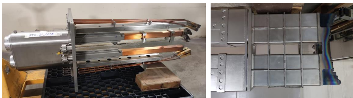
Fig.5: Example of complex objects analysed during the FTU Radiological Pre-Characterization Plan. Left: instrument for reflectometry. Right: diagnostics (heavy steel components).
